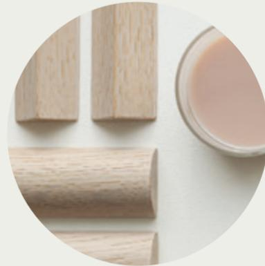
To treat the wood and create a strong, durable surface without the use of solvents or harmful substances, we use an oil composed of linseed-based resins, microcrystalline waxes, zinc, iron, calcium and manganese.
